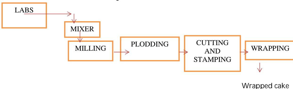
In the process flow sheet, the major raw materials are washing soda; china clay and linear alkyl benzene sulphonates (LABS) which is a acid slurry were in India are fed to the mixer. Later, including surfactants, builders, enzymes are added where each enzyme perform their significant role in for the production of detergent cake. The final process is to the add colour and perfumes and particular or desired shapes are given to detergent cakes.
