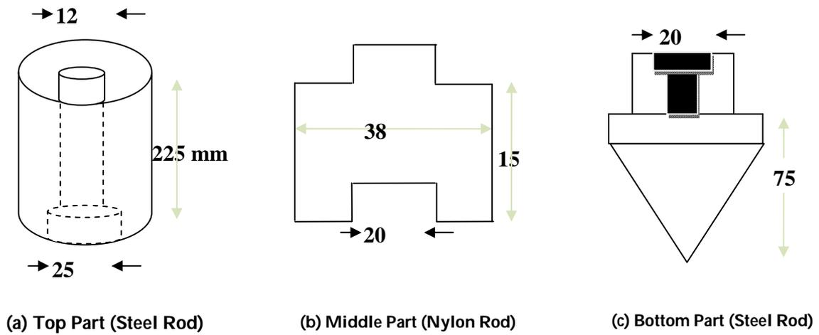
Fig.3. Schematic Diagram of Soil Moisture Sensor
