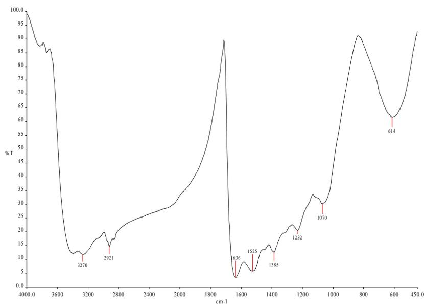
Fig: 4. FTIR spectrum of the silver nanoparticles.
