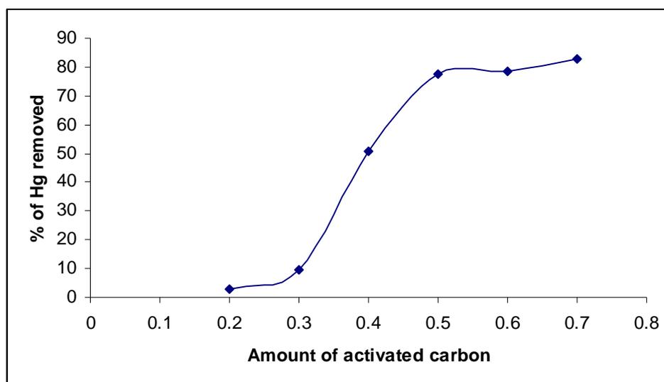
**Fig.3.1: Optimum dosage for activated carbon**
