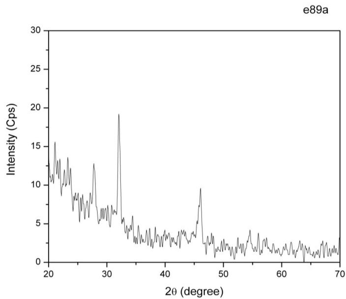
Fig:3 The XRD pattern of the silver nanoparticles
